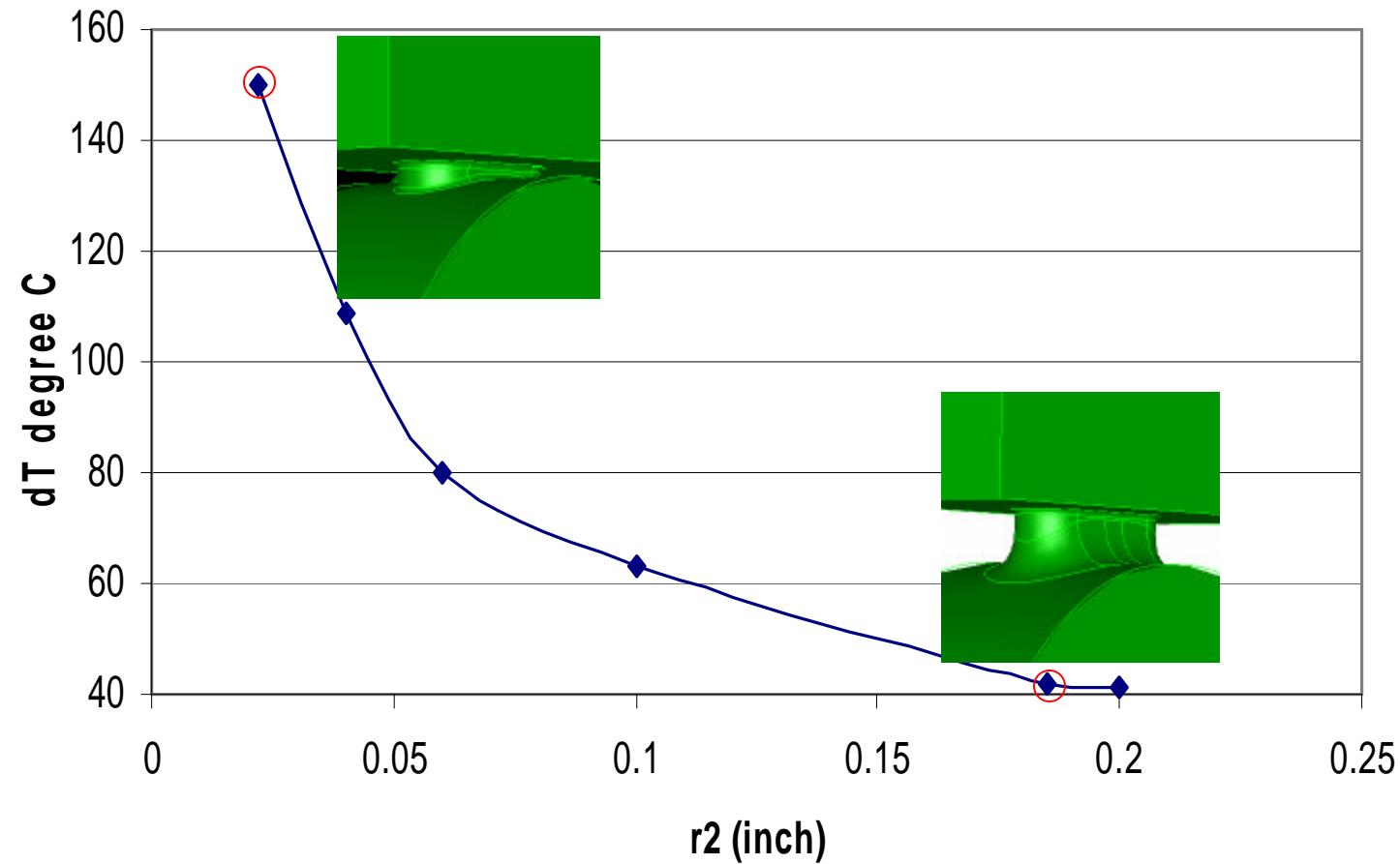
**Temperature rise vs. the rounding radius of the RF aperture**
